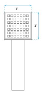
The minimum required water pressure is 0.05 MPa (0.5 bar). Flow rate 2.5 GPM (9.5 LPM).
